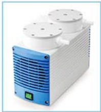
C410 Vacuum pump(18900389) Specifications: Maximum Vacuum:13mbar Work Mode: Continuous Operation Nozzle Size:8mm Power: 95W Motor speed:1450rpm
